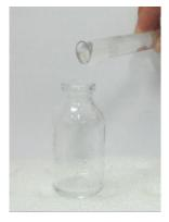
**1.** Fill the tube fully with sample water, then transfer water to the glass bottle.
